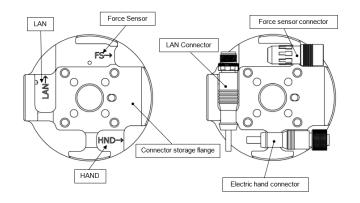
Mounting the connector storage flange
