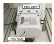
Take out the  $\Phi$ 4 tube and  $\Phi$ 6 tube (white) from the opening
