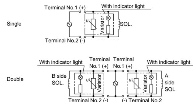
Figure 7. Light/Surge voltage suppressor circuit - AC
