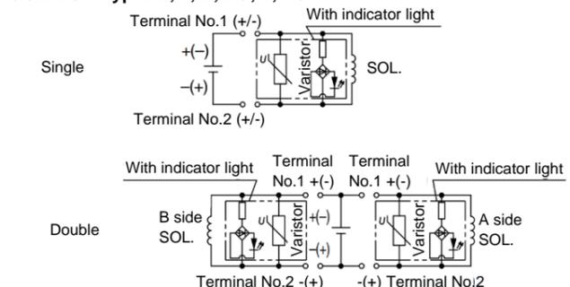
Figure 8. Light/Surge voltage suppressor circuit - DC
