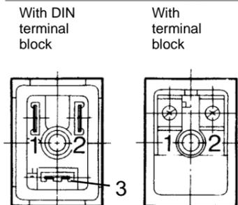
Applicable terminal: 1.25-3, 1.25-3S, 1.25Y-3N, 1.25Y-3S, but in the case of with DIN terminal block, is not a terminal structure.
