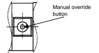
Figure 3. Non-locking push type manual override
