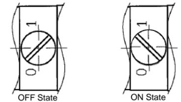
Figure 4. Locking type manual override
