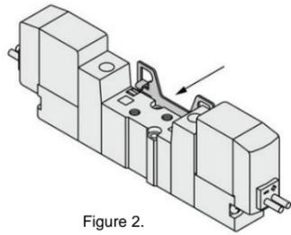
2) Press the valve and mounting bracket together until the upper hook of the bracket snaps into place in the groove on top of the valve.
