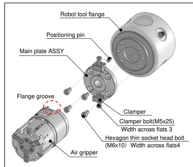
Note: Installation of dedicated flange (identification symbol: 031N, 031P, 041N, 041P, 042N, 042P). Before mounting the main plate ASSY, mount the dedicated flange.
