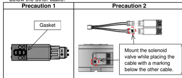
**7.6 Procedure for replacing the solenoid valve (Normally Open, Normally Closed)**
