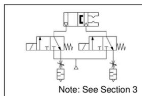
The intended use of this parallel type of air gripper is to convert the potential energy provided by compressed air into a force which causes mechanical linear motion of the fingers.
