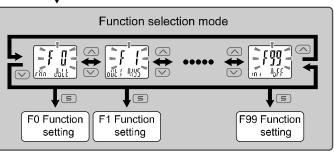
\*: Some products do not have all of the functions. If no function is available or selected due to configuration of other functions, [- - -] is displayed on the sub display (right).
