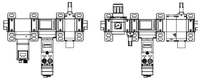
The intended use of the Air Management System is to monitor, control and display flow, pressure and temperature information while connected to a communications protocol.
