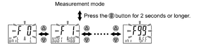
The function number is increased and decreased by the UP and DOWN buttons. Display the required function number and press the SET button.
