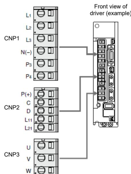
Main circuit power supply connector (CNP1)
