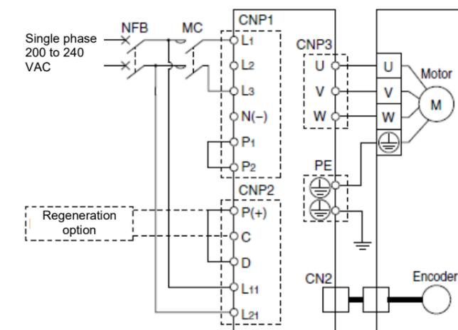
Note) For single phase, the power supply should be connected to terminals L1 and L3 (not L2).
