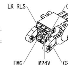
Power supply connector. SMC Part No. JXC-CPW.
