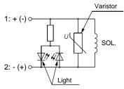
Figure 10. DIN terminal with light and surge voltage suppressor
