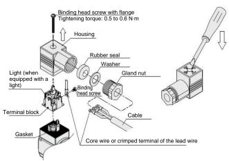
Figure 5. JSX20/30 DIN connector construction
