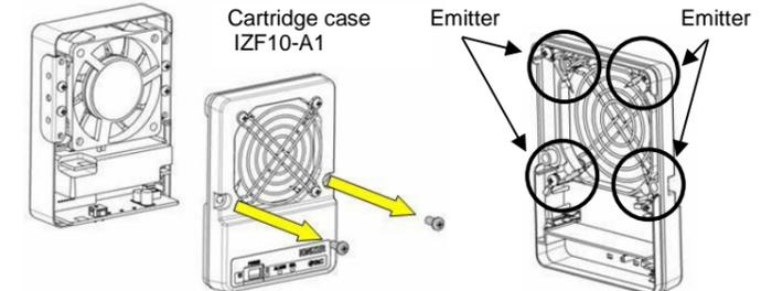
3) 4 emitters are fixed inside the cartridge case. Clean the ends of the emitters. Using the cleaning kit, saturate the felt with industrial alcohol, insert it into the emitters and rotate several times to clean. If the contamination is not removed, use the rubber grindstone to clean the emitters in the same way.
