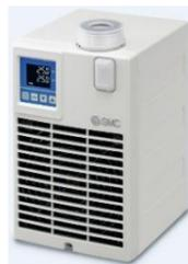
This product used a built-in pump to circulate a liquid (water or 20% EG) at a constant temperature, controlled by Thermo-Electric (Peltier) Modules. This circulating liquid cools parts of customer's machine that generate heat.
