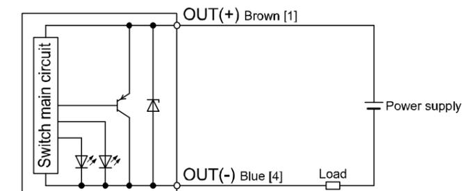
The number shown in brackets [ ] in the wiring diagram indicates the pre-wired connector pin number.
