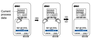
Press the UP or DOWN button to change the set value.The UP button is to increase and the DOWN button is to decrease.Press the SET button once to complete setting the 4th digit and the 3rd
