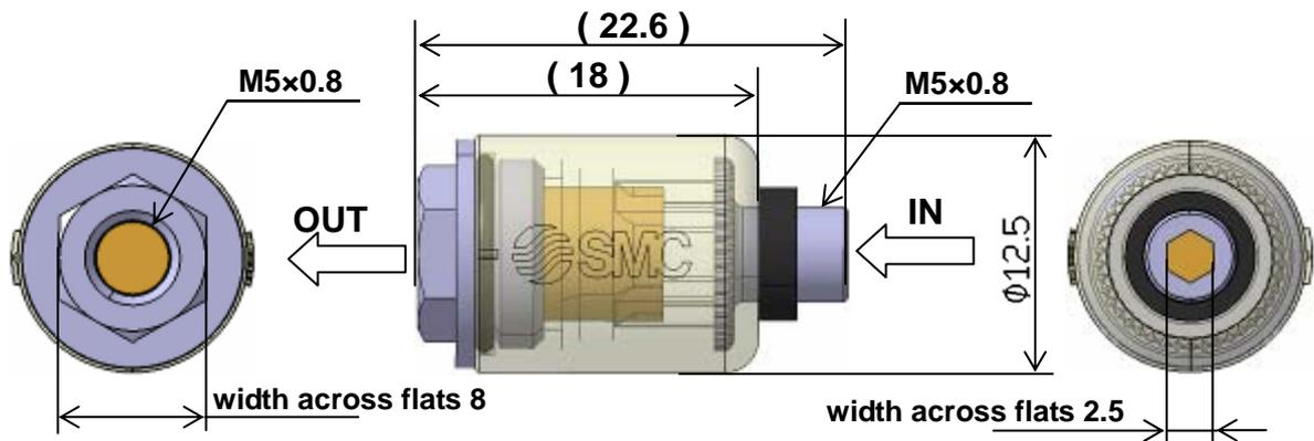
Note 1: Use is possible even with IN-OUT reversed-connection.
