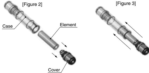
5. Adjust the protrusion on the cover and the slit on the case so that they match up, then push the cover into the end of the case. Next, confirm that the cover is locked by attempting to rotate it clockwise ("O" on the cover ⇔ L marking).
