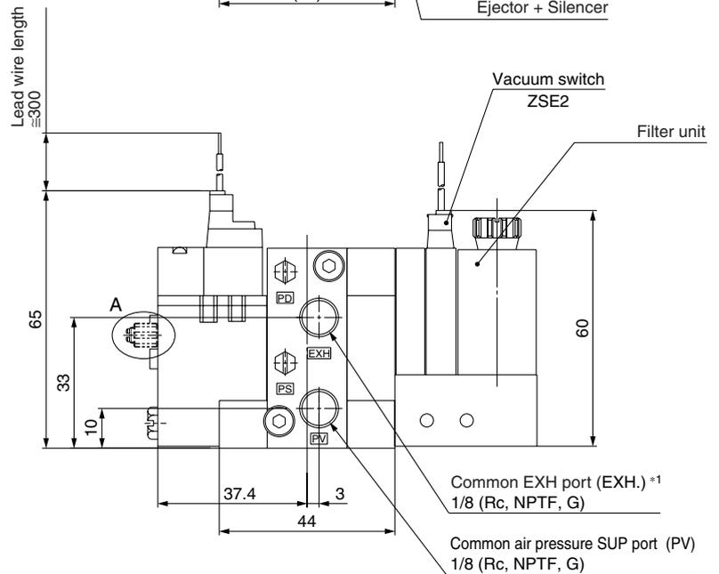
\*1 The common exhaust port (EXH.) is also used as the pilot pressure exhaust (PE) port of pilot valve. Use while the port is open to the atmosphere.
