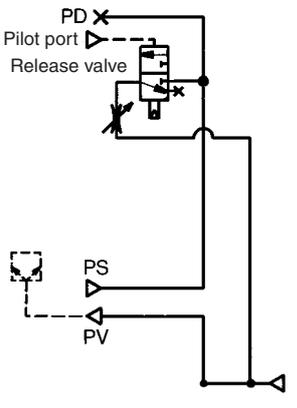
Application: The supply pressure is controlled by the external 2 port valve (vacuum valve) and vacuum release is effected by external air signals.
