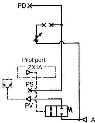
Application: The supply pressure is controlled by external air signals. Normally, the workpiece is released due to the air leakage that occurs between the pad and the workpiece. However, if there is no air leakage, the workpiece will not become detached because the vacuum state is maintained even when the supply valve is turned OFF. To effect releasing, an external 2 port valve (vacuum valve) must be provided.
