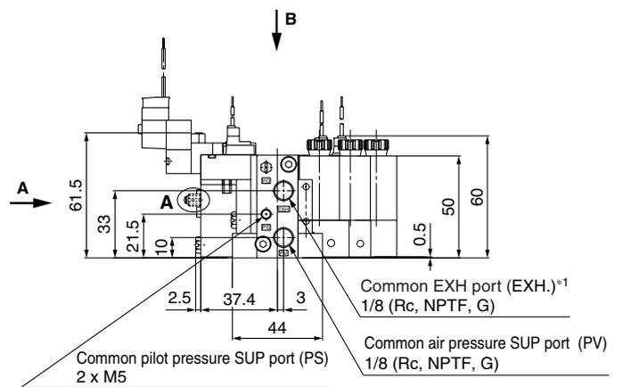
\*1 The common exhaust port (EXH.) is also used as the pilot pressure exhaust (PE) port of pilot valve. Use while the port is open to the atmosphere.
