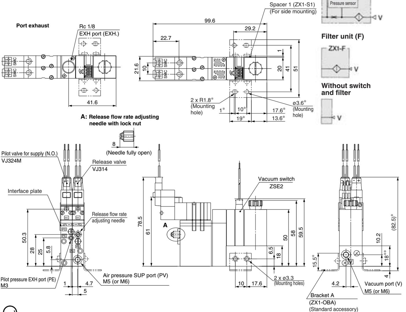
Note) Dimensions \*: For mounting bracket A \*\*: For mounting spacer 1.
