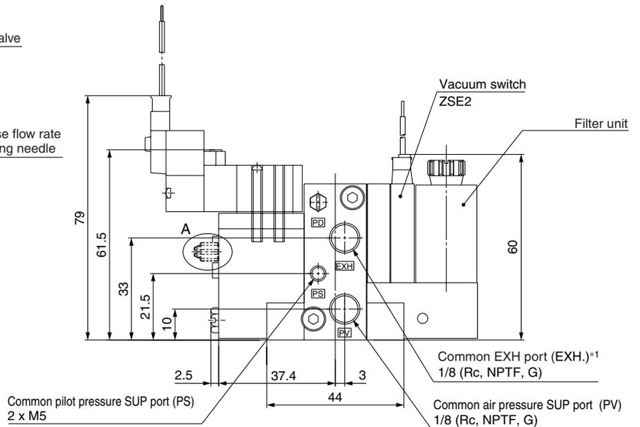
\*1 The common exhaust port (EXH.) is also used as the pilot pressure exhaust (PE) port of pilot valve. Use while the port is open to the atmosphere.
