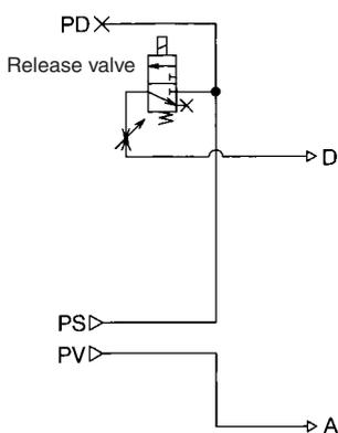
Application: The supply pressure is controlled by the external valve and a vacuum release is effected by the solenoid valve.
