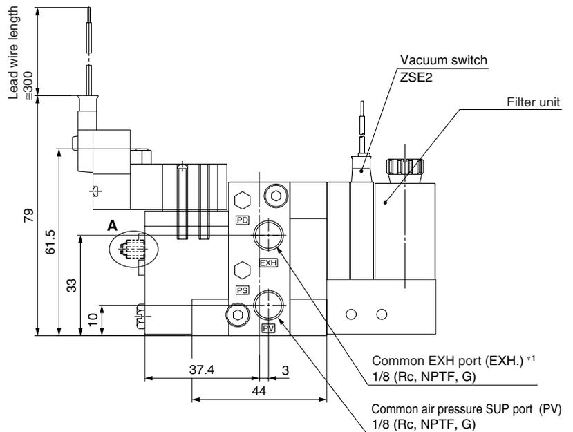
\*1 The common exhaust port (EXH.) is also used as the pilot pressure exhaust (PE) port of pilot valve. Use while the port is open to the atmosphere.
