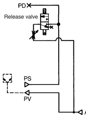
Application: The supply pressure is controlled by an external 2 port valve (vacuum valve) and a vacuum release is effected by the solenoid.
