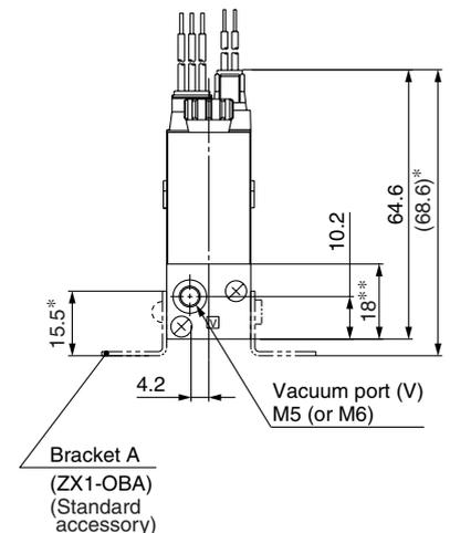
Note) Dimensions \*: For mounting bracket A \*\*: For mounting spacer 1.
