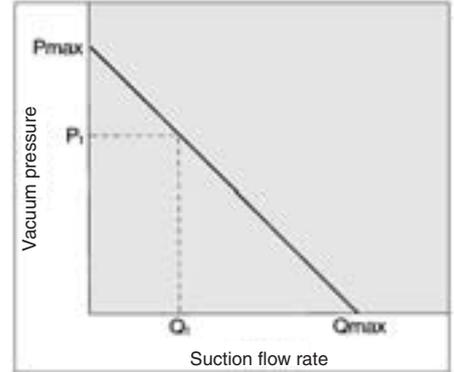
Flow characteristics are expressed in ejector vacuum pressure and suction flow. If suction flow rate changes, a change in vacuum pressure will also be expressed. Normally this relationship is expressed in ejector standard use.
