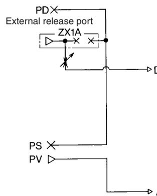
Application: The supply pressure is controlled by the external valve and a vacuum release is effected by the external 2 port valve (vacuum valve).
