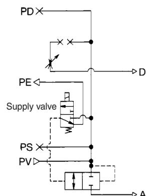
Application: This combination is used for effecting control in accordance with electric signals. A vacuum release is effected by the intrusion of air between the silencer, pad, and the workpiece. This combination is used when there is no need to accelerate the vacuum release speed.
