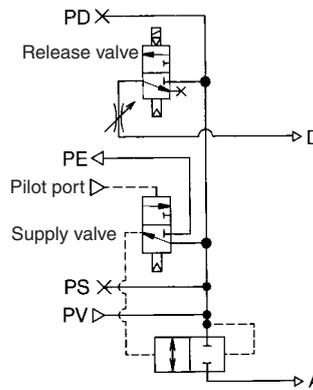
Application: The supply pressure is controlled by external air signals and a vacuum release is effected by the solenoid valve. Because the supply valve is N.O., the pressure that is supplied to the ejector is not interrupted during a power outage; as a result, the state of suction can be maintained. This combination is used for preventing the workpieces from dropping during power outages.
