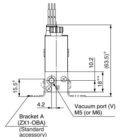
Note) Dimensions \*: For mounting bracket B \*\*: For mounting spacer 2.
