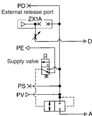
Application: The supply pressure is controlled by electric signals and a vacuum release is effected by external air.
