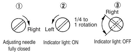
4. Pick a workpiece with the nozzle and readjust the adjusting needle so that the indicator light turns ON when the nozzle has picked the workpiece successfully.
