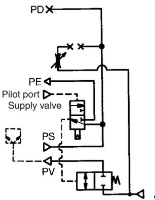
Application: Supply is controlled by external air signals. Because the valve is N.O., the pressure is not interrupted during a power outage. This prevents the workpieces from dropping. Normally, the workpiece is released due to leakage. However, if no leakage, the workpiece will not detach because the vacuum state is maintained even when the valve is turned ON. To release, an external 2 port valve (vacuum valve) must be provided.
