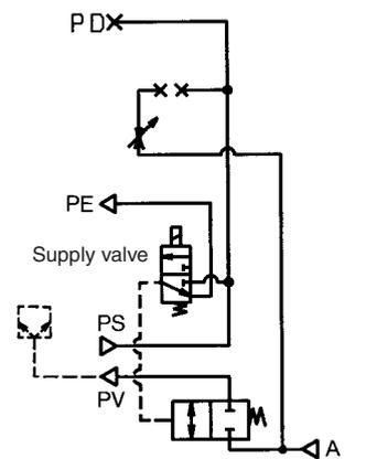
Application: This combination is used for controlling the pressure by electric signals. Normally, the workpiece is released due to the air leakage that occurs between the pad and the workpiece. However, if there is no air leakage, the workpiece will not become detached because the vacuum state is maintained even when the supply valve is turned OFF. To effect releasing, an external 2 port valve (vacuum valve) must be provided.
