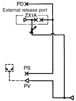
Application: The supply pressure is controlled by the external 2 port valve (vacuum valve) and releasing is also effected by the external 2 port valve.
