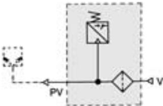
Vacuum Pressure Switch Unit/Adsorption Confirmation Switch: ZSP1-S<sub>B</sub>
