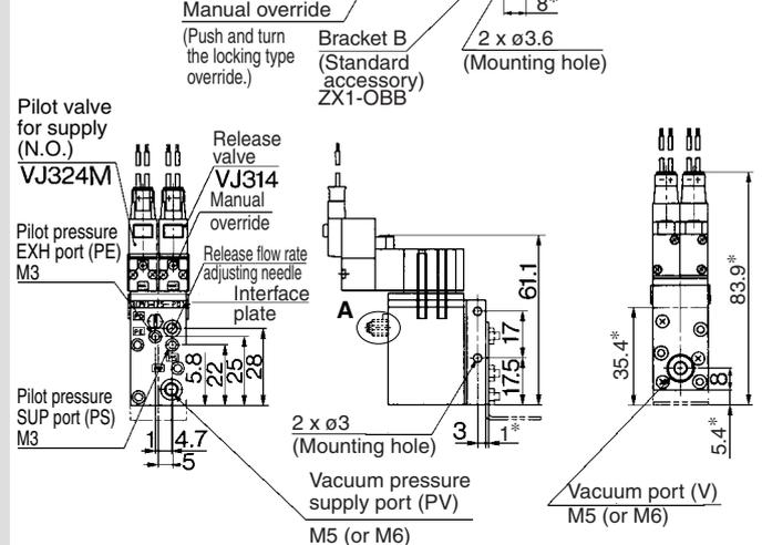
Note) Dimensions \*: For mounting bracket B \*\*: For mounting spacer
