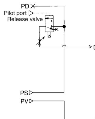
Application: The supply pressure is controlled by the external valve and a vacuum release is effected by external air signals.
