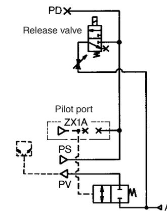
Application: The supply pressure is controlled by external air signals and a vacuum release is effected by the solenoid valve.
