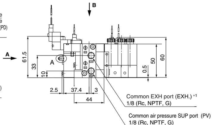
\*1 The common exhaust port (EXH.) is also used as the pilot pressure exhaust (PE) port of pilot valve. Use while the port is open to the atmosphere.
