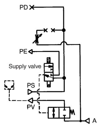
Application: Used for controlling with electric signals. Because the supply N.O., the pressure is not interrupted during a power outage. This prevents the workpieces from dropping. Normally, the workpiece is released due to leakage. However, if no air leakage, the workpiece will not detach because the vacuum state is maintained even when the supply valve is turned ON. To release, an external 2 port valve (vacuum valve) must be used.
