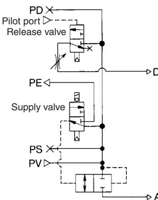
Application: The supply pressure is restricted by electric signals and a vacuum release is effected by air signals. Because the supply valve is N.O., the pressure that is supplied to the ejector is not interrupted during a power outage; as a result, the state of suction can be maintained. This combination is used for preventing the workpieces from dropping during power outages.
