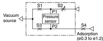
The air pressure forms a bridge circuit inside the unit with a vacuum applied to the circuit, but with the adsorption nozzle "S4" open, adjust needle "S2" so that (P1 = P2). When parts are absorbed by nozzle "S4", the resulting (P2 - P1) differential will be detected by the pressure sensor.
