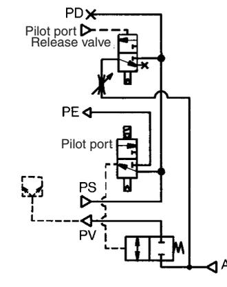
Application: The supply pressure is controlled by electric signals and a vacuum release is effected by air signals. Because the supply valve is N.O., the pressure that is supplied to the ejector is not interrupted during a power outage; as a result, the state of suction can be maintained. This combination is used for preventing the workpieces from dropping during power outages.
