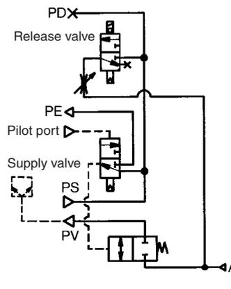
Application: The supply pressure is controlled by external air signals and a vacuum release is effected by the solenoid valve. Because the supply valve is the N.O., the pressure that is supplied to the ejector is not interrupted during a power outage; as a result, the state of suction can be maintained. This combination is used for preventing the workpieces from dropping during power outages.
