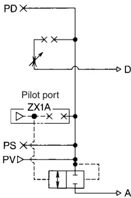
Application: The supply pressure is controlled by external air signals. A vacuum release is effected by the intrusion of air between the silencer, pad, and the workpiece. This is used when there is no need to accelerate the vacuum release speed.
