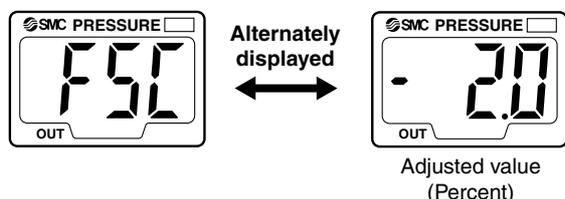
Press the SET button to return to the normal measuring mode.
