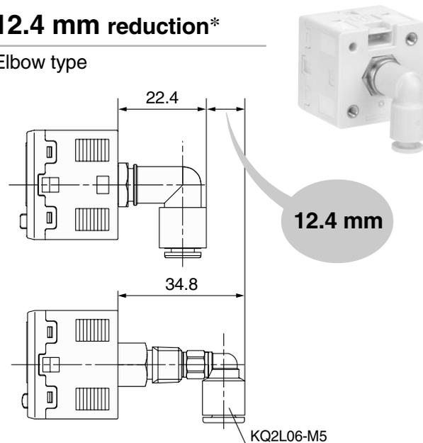
\* Comparison when One-touch fittings (KQ2H06-M5 / KQ2L06-M5) are connected to the piping ports (M5 x 0.8)
