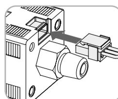
Plug-type connectors take the burden out of wiring work and maintenance.
