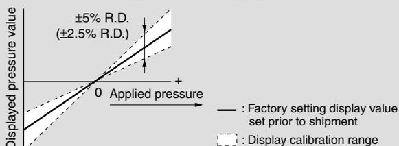
Note) When the display calibration function is used, the regulating pressure value may change  $\pm 1$  digit.
