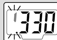
4. Press and hold the SET button for 1 second or longer to return to the set value display mode.
