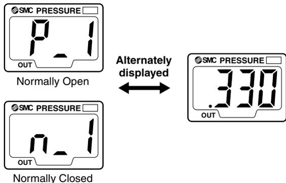
Press the SET button to display the next set value. Press the  $\Delta$ UP or  $\nabla$ DOWN button to change the value. (Refer to "How to Set Value" on the lower right hand corner of this page.)
