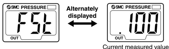
Press the SET button to display the adjusted value (percent). The adjusted value and F5L will be alternately displayed.
