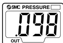
This function eliminates slight differences in the output values and allows uniformity in the numbers displayed. Displayed values of the pressure sensor can be calibrated to within  $\pm 5\%$  for Series ISE and  $\pm 2.5\%$  for Series ZSE.
