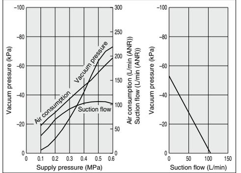
**ZR1-W13L1 Exhaust characteristics**      **Flow characteristics**
