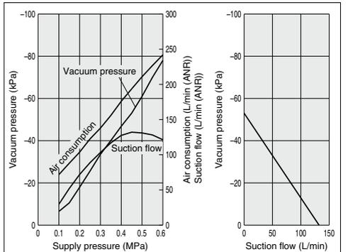
**ZR1-W15L1 Exhaust characteristics**      **Flow characteristics**
