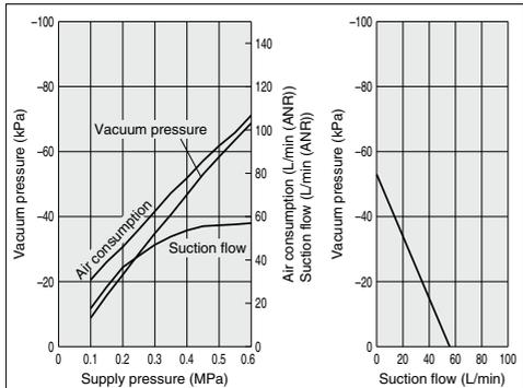
**ZR1-W20L1 Exhaust characteristics**      **Flow characteristics**
