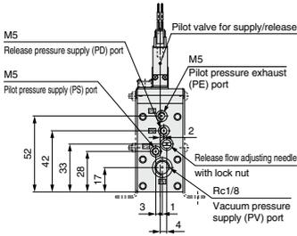
**A: Release flow adjusting needle with lock nut**
