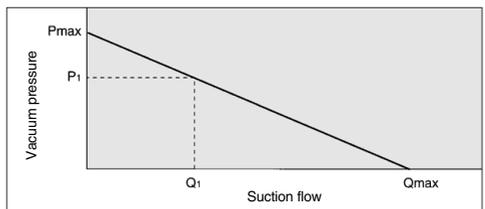
Flow characteristics are expressed in ejector vacuum pressure and suction flow. If suction flow rate changes, the vacuum pressure will also be changed. Normally this relationship is expressed in ejector standard use. In graph, Pmax is max. vacuum pressure and Qmax is maximum suction flow. The values are specified according to catalog use. Changes in vacuum pressure are expressed in the below order.
