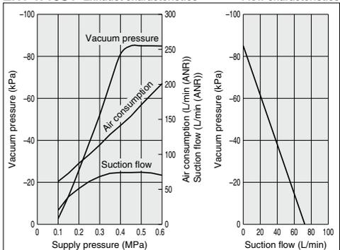
ZR1-W13S1 Exhaust characteristics Flow characteristics
