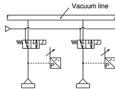
When pads and switches are common to one vacuum source, sometimes there is a possibility, depending on the number of adsorption and non-adsorption applications at each point in time, that the switches will not work within the range of set pressures due to pressure variations from the vacuum source. In particular, when small diameter nozzles are used for adsorption, the switches are greatly influenced by pressure variations. In order to remedy this situation, the following circuit is recommended.
