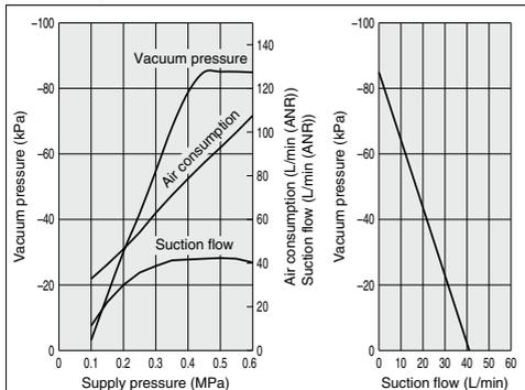
ZR1-W20S1 Exhaust characteristics Flow characteristics
