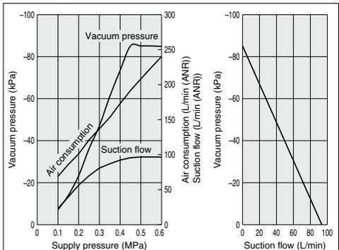
ZR1-W15S1 Exhaust characteristics Flow characteristics
