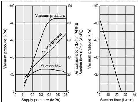
ZR1-W18S1 Exhaust characteristics Flow characteristics
