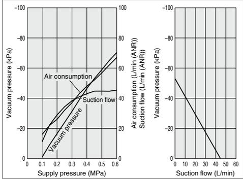
**ZR1-W18L1 Exhaust characteristics**      **Flow characteristics**
