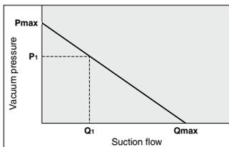
Flow rate characteristics are expressed in ejector vacuum pressure and suction flow. If suction flow rate changes, a change in vacuum pressure will also be expressed. Normally this relationship is expressed in ejector standard use.
