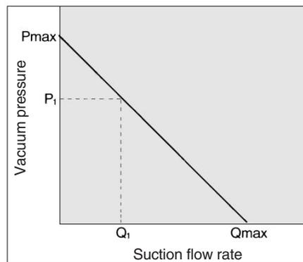
Flow characteristics are expressed in ejector vacuum pressure and suction flow. If suction flow rate changes, a change in vacuum pressure will also be expressed. Normally this relationship is expressed in ejector standard use.
