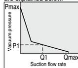
1. If the ejector's suction port is closed and sealed tight, the suction flow rate becomes "0" and the vacuum pressure increases to the maximum (Pmax).
