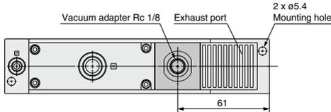
**With digital pressure switch for vacuum
