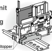
Manifold DIN rail mounting
