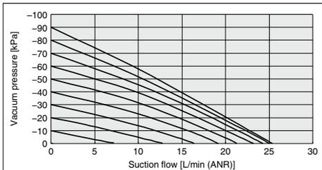
The actual suction flow at the point of suction varies depending on the piping conditions to the vacuum port. (The above graph shows the value when V port is ø8.)
