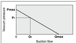
Flow rate characteristics are expressed in ejector vacuum pressure and suction flow. If suction flow changes, the vacuum pressure will also be changed. Normally this relationship is expressed in ejector standard operating pressure use. In graph, **Pmax** is maximum vacuum pressure and **Qmax** is maximum suction flow. The values are specified according to catalog use. Changes in vacuum pressure are expressed in the below order.
