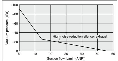
**Ejector Exhaust Characteristics/Flow Rate Characteristics (Representative value)**
