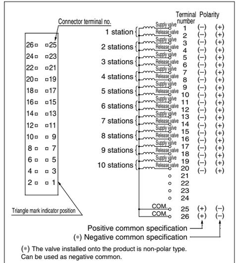
A D-sub connector (25P) conforming to MIL standards is used.
