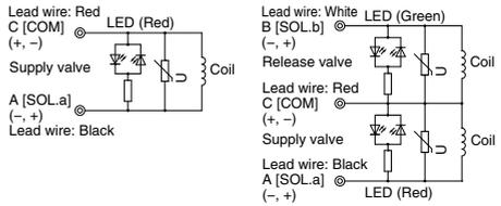
Light/surge voltage suppressor circuit is equipped for both single and double solenoid. Red LED turns on when supply valve (SOL.a) is energized. Green LED turns on when release valve (SOL.b) is energized.
