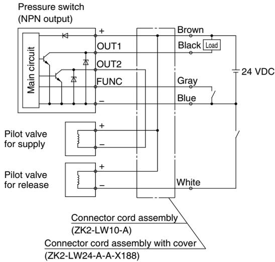
For pressure switch for vacuum with energy-saving function:
