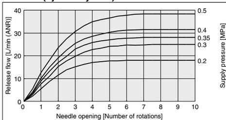
The actual suction flow at the point of suction varies depending on the piping conditions to the vacuum port. (The above graph shows the value of the ZK2B07.)
