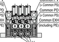
Note) The complex exhaust is a combined exhaust method of the common exhaust from the end plate and the direct exhaust from each station.
