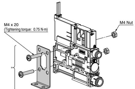
\*Mounting bracket for single unit (Option), [Nuts and bolts are included.]
