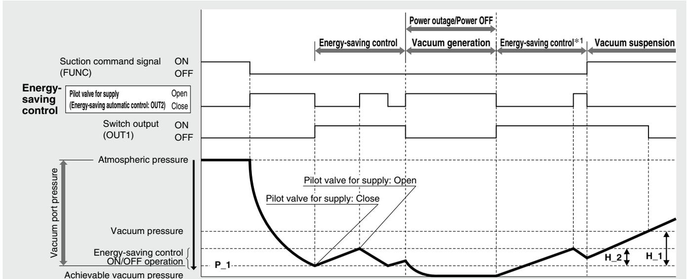
\*1 A minute after the power supply is turned on again, the energy-saving control and the switch's output (OUT1) are initiated.
