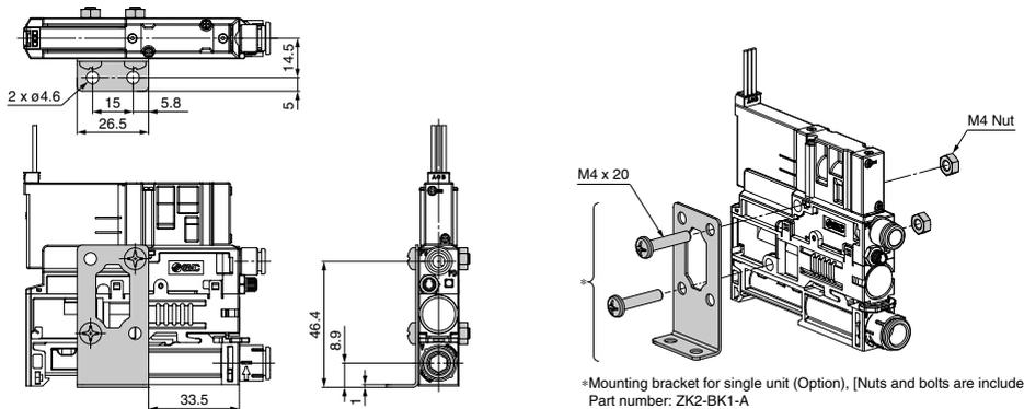
\*Mounting bracket for single unit (Option), [Nuts and bolts are included.]
