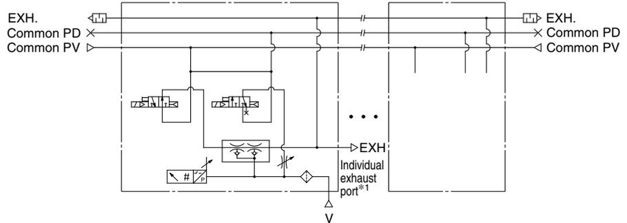
\*1 For the complex exhaust type, an individual exhaust port is provided to each station.
