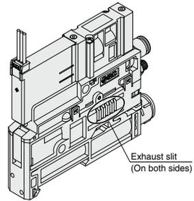
For port exhaust type, back pressure may increase depending on the piping size and length. Ensure that the back pressure does not exceed 0.005 MPa (5 kPa).
