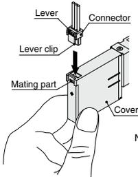
Note) Do not pull the lead wire with a force of 25 N or more, as this may damage the connector or cover.
