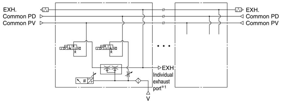
\*1 For the complex exhaust type, an individual exhaust port is provided to each station.
