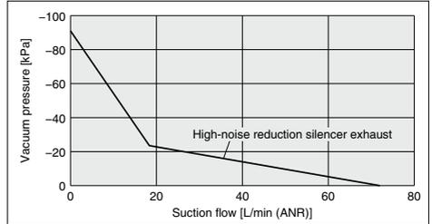
**ZK2□15** Note 8) The following graphs show the characteristics of the ejector with valve. (Please contact SMC for models without valve.)
