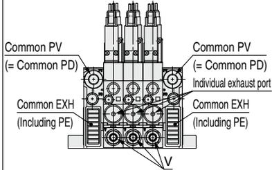
\*1 The complex exhaust method combines the common exhaust from the end plate and the direct exhaust from each station.
