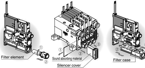
• Transparent filter case allows visual check of the contamination.
