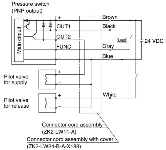
\* The pressure switch for vacuum with energy-saving function and the connector cord assembly with cover are the same for both the ZK2□A-X188 and the ZK2□A-X211.
