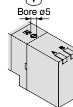
Push down the manual override button with a small flat head screwdriver until it stops, and turn it clockwise 90° to lock it. Turn it counterclockwise to release it.
