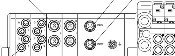
**Input connection: M8 ... 3 pins (Socket)**
