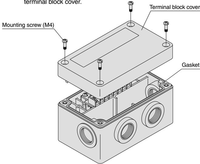
**Step 2. Wire the cables according to the terminal block specifications below. Pay attention to the wire bound positions.**
