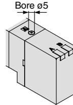
Push down the manual override button with a small screwdriver until it stops. The manual override will return when released.
