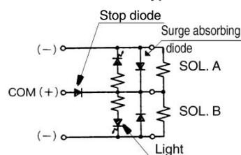
With miswiring prevention mechanism (stop diode)
