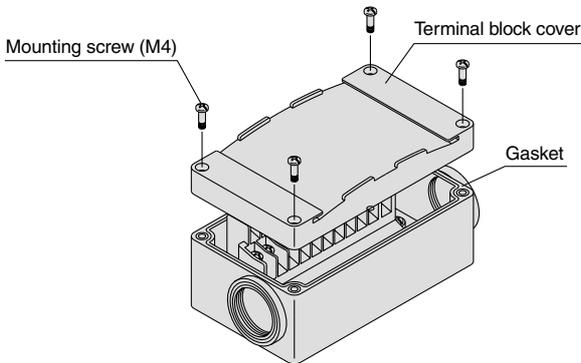
**Step 3. How to replace the terminal block cover**
