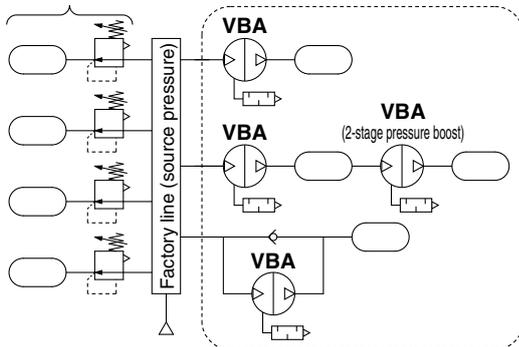
\* When using 2 booster regulators for 2-stage pressure boost, be sure to supply sufficient flow to each booster regulator in order to stabilize the booster regulator inlet pressure. Refer to "Selection 2" on page 11 for the inlet side supply amount.
