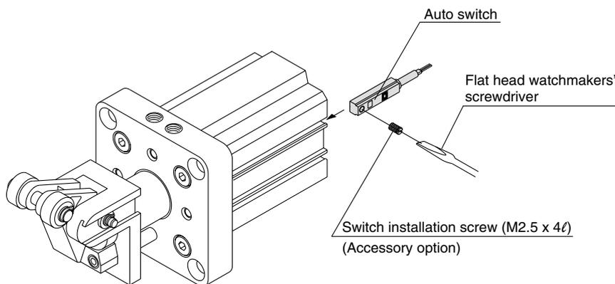
Note) When adjusting the auto switch mounting screws, use a flat head watchmakers' screwdriver. The guideline of the tightening torque is 0.05 to 0.1 Nm. Turn another 90° from the position where tightening is felt by hand.
