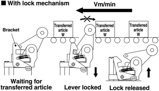
A repulsion preventing mechanism keeps light pallets, etc., from being pushed back by the reactive force of the shock absorber's spring.
