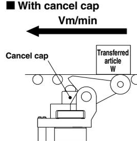
The lever is set to a pallet pass position allowing some pallets to pass by.
