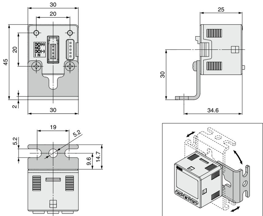
\* Bracket configuration allows for mounting in four orientations.
