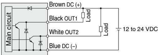
Max. applied voltage: 30 V, Max. load current: 80 mA, Internal voltage drop: 1.5 V or less
