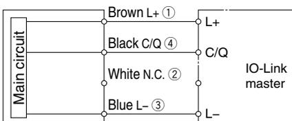
\* The numbers in the diagrams show the connector pin layout.
