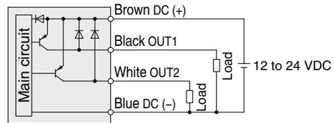
Max. load current: 80 mA, Internal voltage drop: 1.5 V or less
