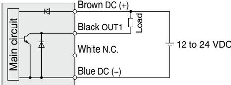
Max. applied voltage: 30 V, Max. load current: 80 mA, Internal voltage drop: 1.5 V or less
