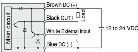
Max. applied voltage: 30 V, Max. load current: 80 mA, Internal voltage drop: 1.5 V or less
