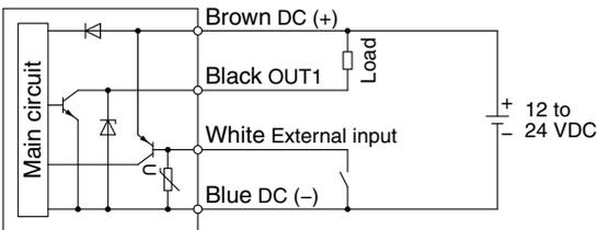
Max. applied voltage: 28 V, Max. load current: 80 mA, Internal voltage drop: 1 V or less
