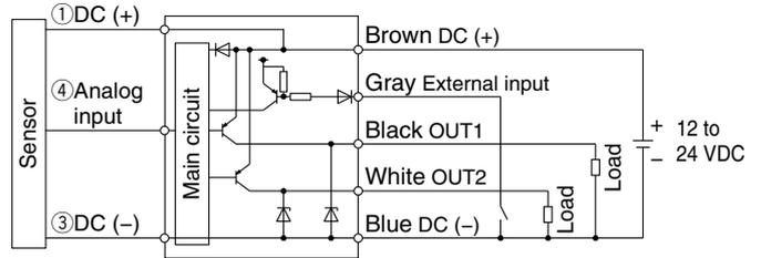
**Accumulated pulse output wiring examples**
