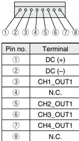
**Power supply / Output connector (accessory)**
