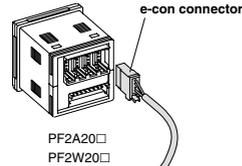
In addition to the lead wire assembly shown above, those listed below (female contact) can be connected. However, they cannot be connected with an e-con connector because the diameter of the core wire and its coverage diameter are different. For details, contact each manufacturer. Contact each manufacturer for details including RoHS compliance.
