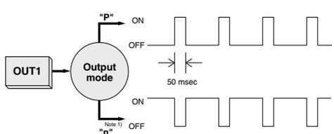
Note 1) Refer to the specifications of monitor unit for the flow rate value per pulse.
