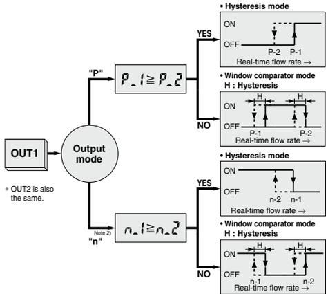
Note 2) Output mode is set to inverted output at the factory before shipment.
