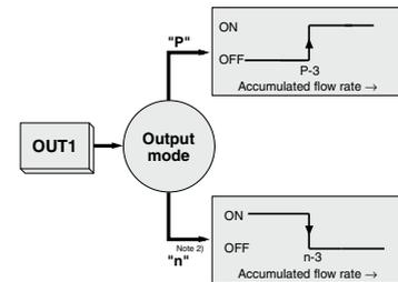
Note 2) Output mode is set to inverted output at the factory before shipment.
