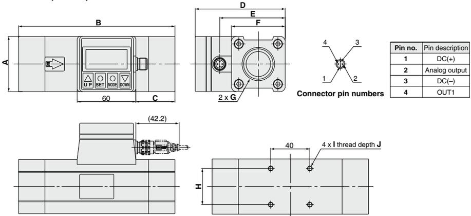
Be sure to allow straight pipe length that is minimum 8 times the port size upstream and downstream of the switch piping.
