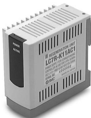
The regenerative absorption unit absorbs the energy (regenerative energy) that is generated by the motor when it decelerates. It is used to prevent drive power abnormality in the controller.
