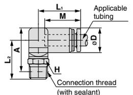
\* Reference dimensions after installation of R thread
