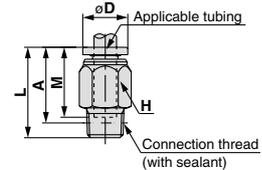
\* Reference dimensions after installation of R thread
