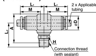
\* Reference dimensions after installation of R thread
