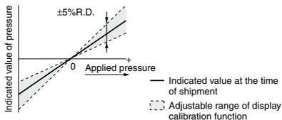
Note) When the display calibration function is used, the set pressure value may change  $\pm 1$  digit.
