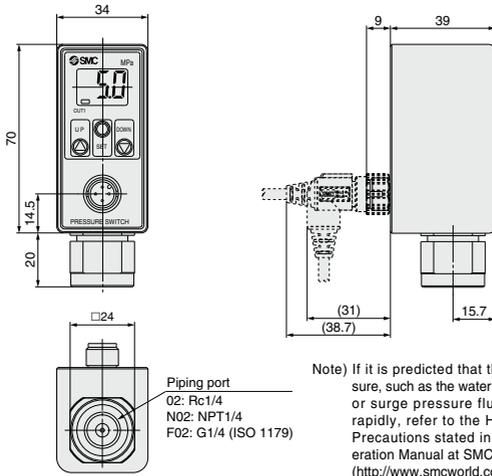
Note) If it is predicted that the pressure, such as the water hammer or surge pressure fluctuates rapidly, refer to the Handling Precautions stated in the Operation Manual at SMC website (<http://www.smcworld.com>).
