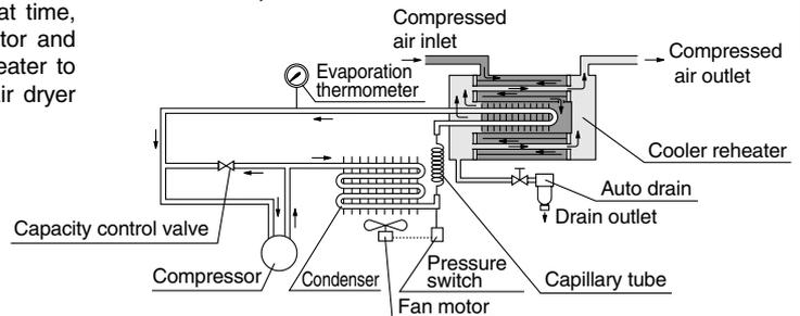
Hot humid air entering the air dryer is cooled by the cooler. At that time, condensed moisture is separated from the air by the drain separator and automatically discharged. The dried clean air is heated by the reheater to about the ambient temperature, and is then discharged from the air dryer outlet.
