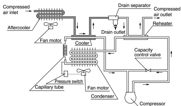
Humid hot air entering the air dryer is cooled in the aftercooler (air-cooling style) and then further cooled by the cooler.
