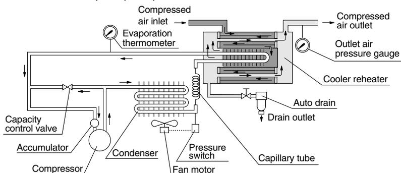
Hot humid air entering the reheater is pre-cooled by dehumidified cool air. (The hot air is cooled further and dehumidified inside the cooler as heat is transferred to the refrigerant. The water condensed by the cooling process is collected and discharged automatically by the auto drain.) Finally, the cool dehumidified air is heated in the reheater by hot inlet air and discharged in a dry state.
