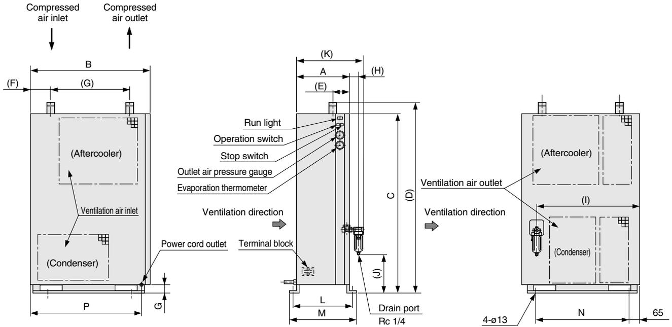
\* Auto drain is packed together with air dryer. (Some assembly is required.)
