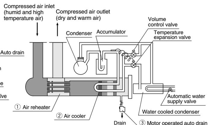
High temperature humid air is cooled in the reheater ①. Then it is further cooled to a specified temperature using the evaporation heat in the air cooler ②. The oil mist and moisture occurring due to condensation is exhausted through the auto drain ③. Cooled and dehumidified air is returned to the air reheater ① and heat is transferred from the incoming high temperature air. It is then exhausted out of the air dryer as dry air.
