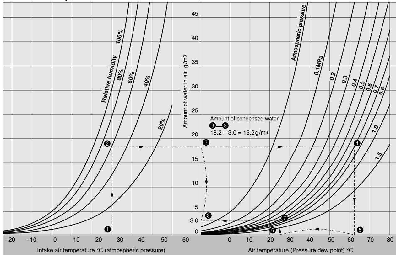
[Example] If air at 30°C and 60% humidity is pressurized to 0.7MPa, the dew point of the air will be 62°C. (1→2→3→4→5) If this is cooled to 25°C, the amount of condensed water generated will be 15.2g/m<sup>3</sup>. (6→7→8→9) Therefore, with an air flow rate of 3m<sup>3</sup>/min (22kW equivalent compressor), the amount of condensed water per unit of time is 15.2 x 3 x 60 = 2736g/h.
