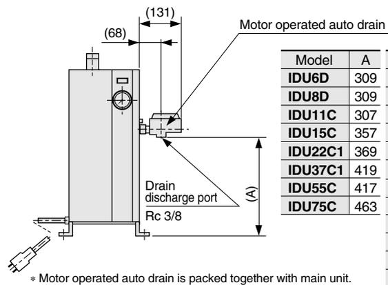
\* Motor operated auto drain is packed together with main unit. Assembly is required.
