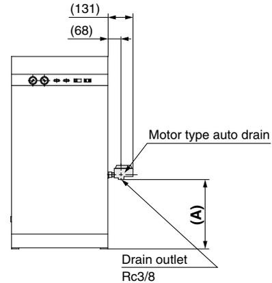
\* The motor type auto drain is enclosed in the same shipping package as the main body of the air dryer. Customers are required to mount the auto drain to the air dryer.
