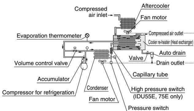
Humid, hot air coming into the air dryer will be cooled down by a heat exchanger. Water condensed at this time will be removed from the air by a drain separator and drained out automatically. Air separated from the water will be heated by a heat exchanger to obtain the dried air, which goes through to the outlet side.
