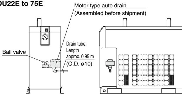
\* When a longer drain tube than the one attached is necessary, remove and replace it with a tube prepared by customers.
