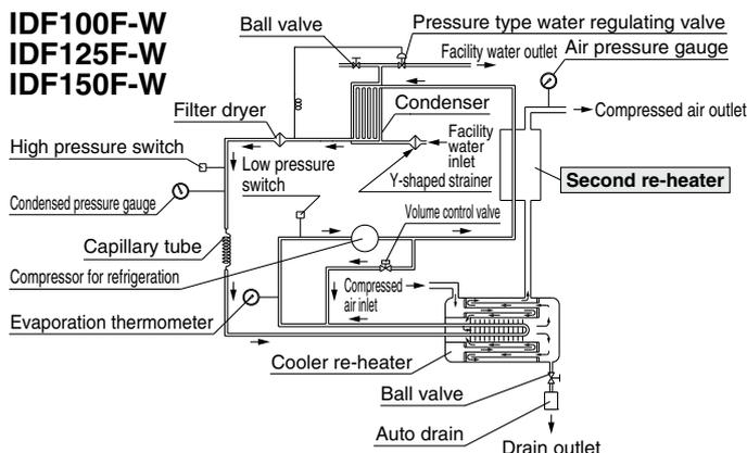
Hot and humid air entering the air dryer is cooled down by the cooler re-heater (heat exchanger). The moisture which is condensed and separated is automatically exhausted by the auto drain. The air which has had its moisture removed is heated in two stages by the re-heater (heat exchanger) in the cooler re-heater and by the second re-heater, and is supplied to the outlet side as warm and dry air.
