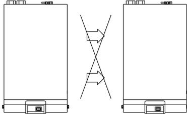
Confirm that the exhaust air does not flow into the neighboring equipment.
