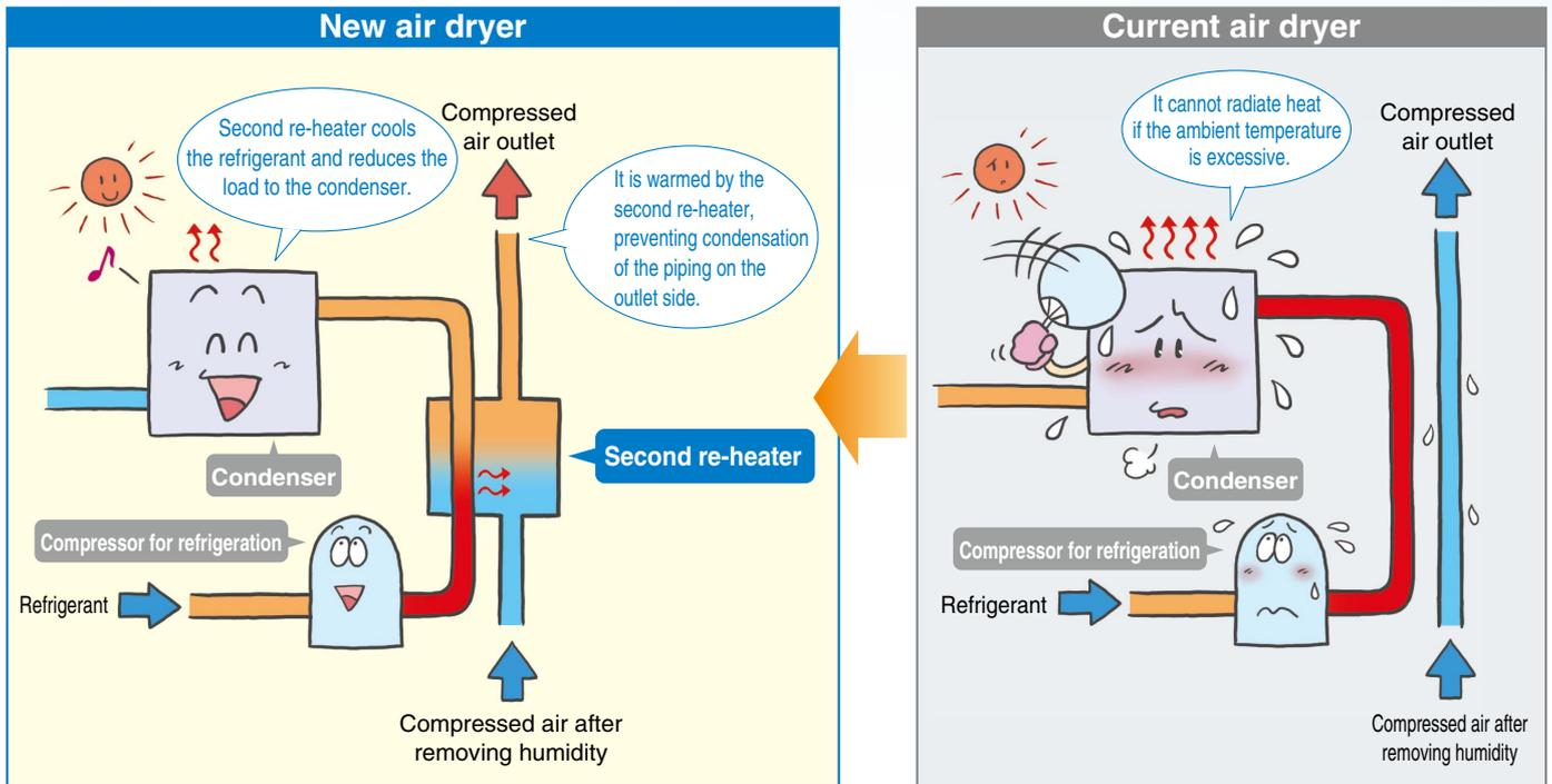
**Energy saving design: Reduces exhaust heat from air dryer by up to 25%.**
