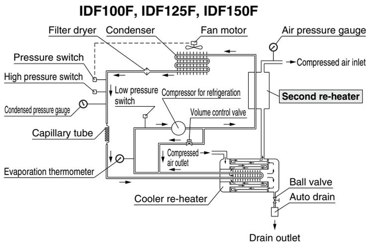
Hot and humid air entering the air dryer is cooled down by the cooler re-heater (heat exchanger). The moisture which is condensed and separated is automatically exhausted by the auto drain. The air which has had its moisture removed is heated in two stages by the re-heater (heat exchanger) in the cooler re-heater and by the second re-heater, and is supplied to the outlet side as warm and dry air.
