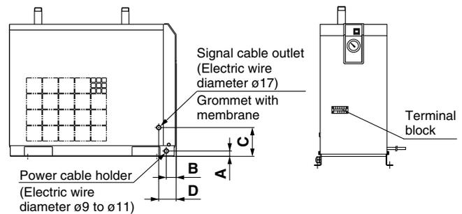
Contact capacity: Operating signal ... 220 VAC, 6 A
