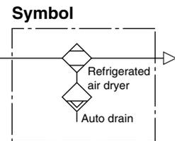
High temperature humid air from the air compressor passes through the air re-heater ① and is pre-cooled by dehumidified cool air. Then, it is cooled to the specified temperature by the air cooler ② using the evaporation heat of refrigerant.
