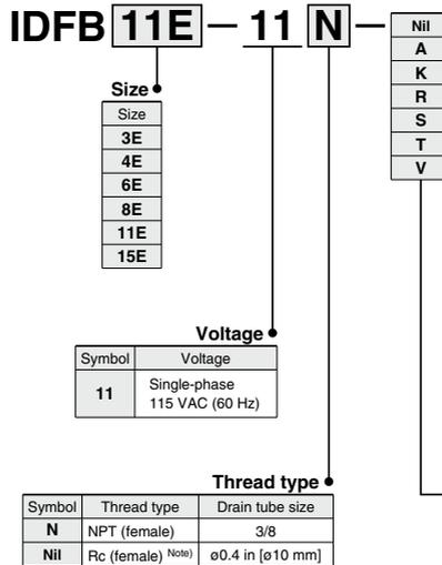
Note) An adapter for converting NPT to Rc is included if the thread symbol is "Nil".
