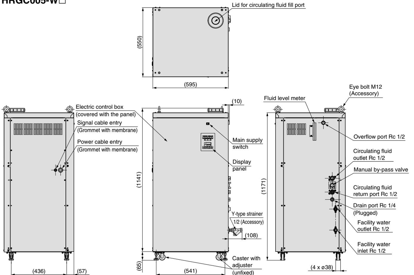
Y-type strainer and eye bolts included. (Not assembled)
