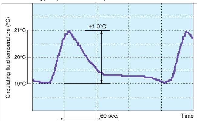
Note 3) The value shown applies to a stable load state with no outside interference.
