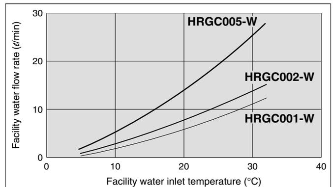
\* This is the flow rate of facility water at the rated cooling capacity and circulating fluid flow, operating at 60 Hz.
