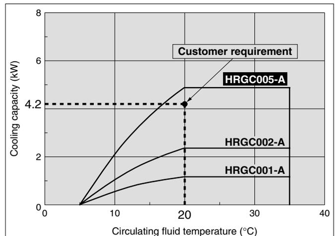
The point plotted in the graph is the requirement from your customer. Select the Thermo-cooler models exceeding this point. In this case, select the **HRGC005-A**.
