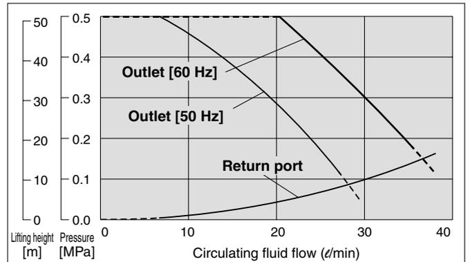
\* For all common models, temperature stability will decline in the flow rate range where circulating fluid is deduced (dotted line).
