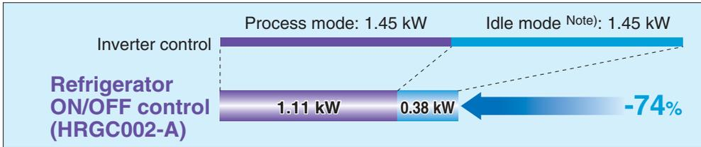
Note) Operating conditions: Process mode: Circulating fluid temperature 20°C, Heat load 2 kW
