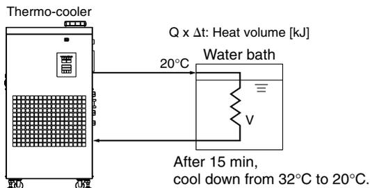
Note) This is the calculated value by changing the fluid temperature only. Thus, it varies substantially, depending on the water bath or piping shape.
