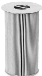
A cylindrical element in which the non-woven material made of P.P. (Polypropylene) is sandwiched by a PET mesh and pleated.
