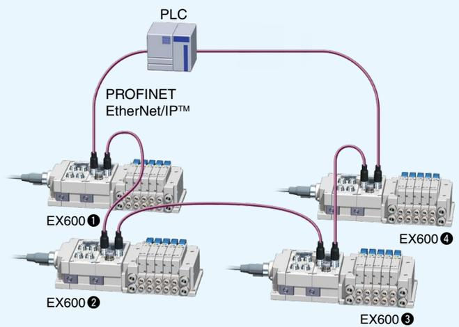
For ring networks, communication can be continued even if one of the communication cables in the network is disconnected or damaged. As the EX600-SEN3/4 supports Device Level Ring (DLR), and the EX600-SPN3/4 supports Media Redundancy Protocol (MRP), the disconnected point can be identified.
