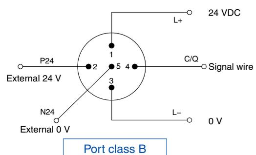
The control power supply wire, external power supply wire, and signal wire can be connected with one cable. (Mainly for actuators)
