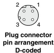
Plug connector pin arrangement D-coded
