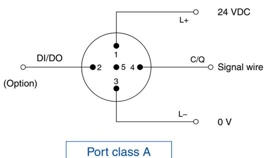
The control power supply wire and signal wire can be connected with one cable. (Mainly for sensors)
