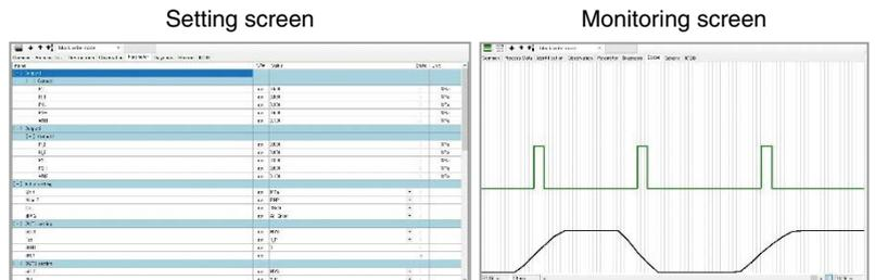
The setting and monitoring of the master and device are possible via PC, without using the PLC.
