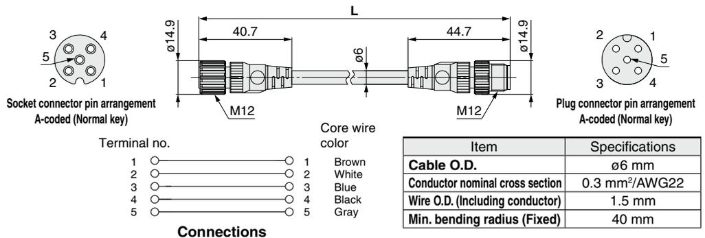
**13 I/O Cable with Connector, I/O Connector**
