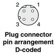
Plug connector pin arrangement D-coded
