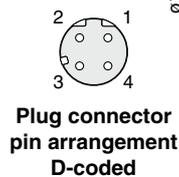
Plug connector pin arrangement D-coded
