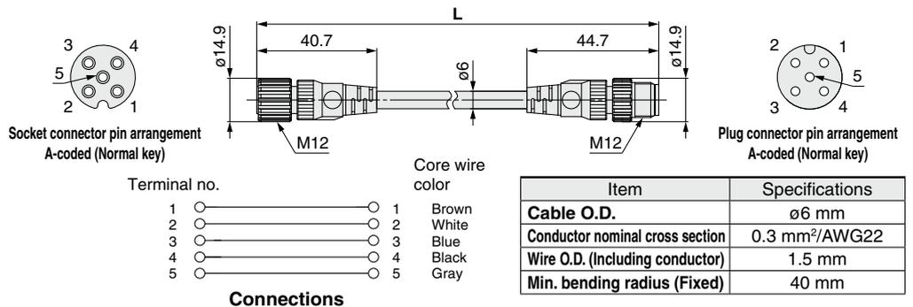
**13 I/O Cable with Connector, I/O Connector**
