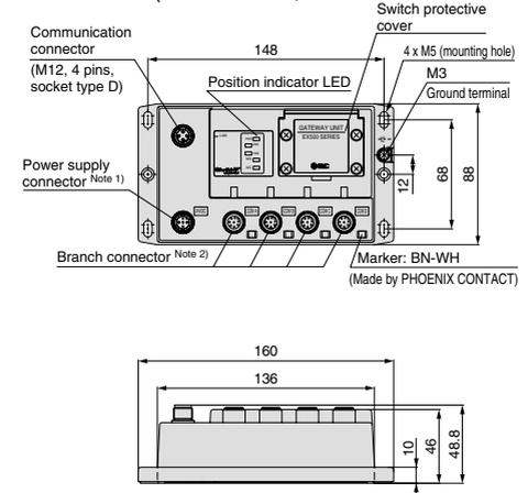
Note 1) Power supply connector specification (M12, 5 pins, plug)
