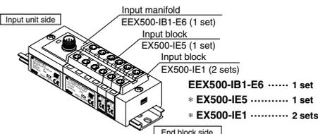
Note • Since the 8 points integrated type input block is equivalent to the length of four stations on an M8 input block, pay attention to the number of stations on an input manifold.
