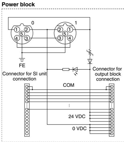
\* When the valve which supplies power to the SI unit is turned OFF, the output of the output block (EX9-OE□) remains OFF.
