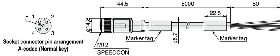
Socket connector pin arrangement
