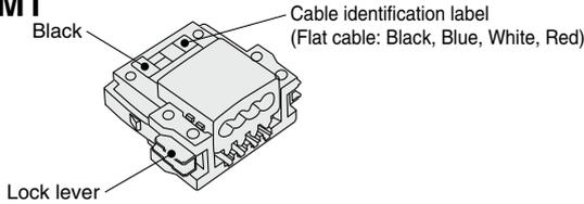
Terminal block connector for round cables (VCTF)
