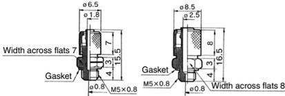
In addition to the above fittings and hose nipples, the below fittings can also be attached to the cylinder. When using the below fittings be sure to provide a speed controller after adjusting it to 500 mm/s or less.
