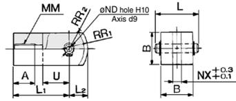
\* Knuckle pin and retaining ring are included.
