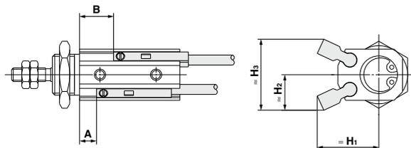
Applicable Auto Switches: D-A9□, D-A9□V
