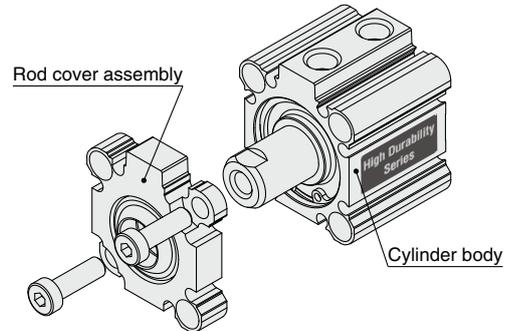
**2. Apply grease to the surface of the piston rod, and install the new rod cover assembly without scratching the Lube-retainer or scraper.**
