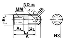
Material: Free cutting sulfur steel (mm)
