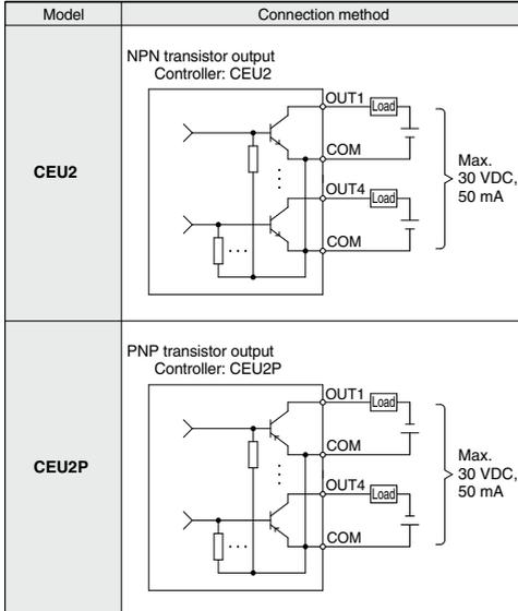
\* However, on the valve output side, the COM of the input circuit and the COM of the output circuit are electrically insulated from each other.
