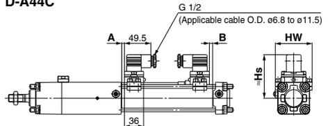
**Auto Switch Proper Mounting Position (Detection at Stroke End) and Its Mounting Height**
