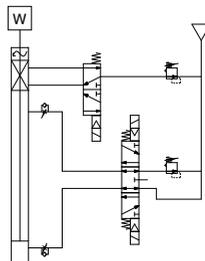
Note) In the case of light load, regulate head side supply pressure.
