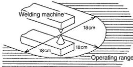
The sensor unit is adjusted to an appropriate position at the time of shipment. Therefore, never detach the sensor unit from the body. Make sure that water does not splash on the sensor unit (enclosure IP65). Do not pull on the sensor cable.
