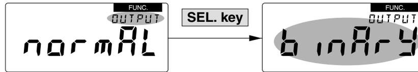
• The output system setting mode is selected by pressing the SEL. key while OUTPUT is flashing.
