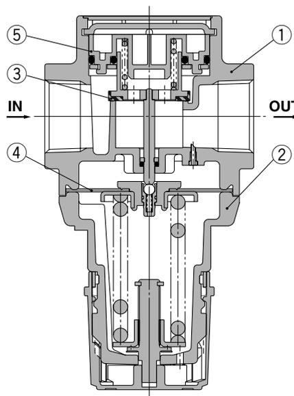
**AR20K to AR60K (Regulator with Backflow Function)**
