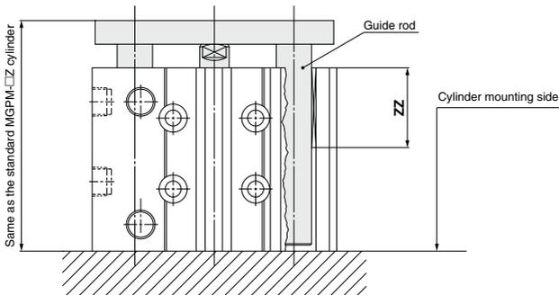
(Note) The total length (ZZ) of the guide rod bushing is shorter than the standard type.
