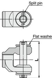
Clevis pin/Knuckle joint pin
