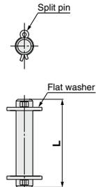
\* Body mounting bolts, pin, split pins, and flat washers are included.
