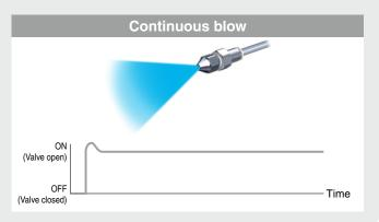
Control for pulse generation is not required. Pulse blow can be used by simply supplying air.
